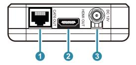
**1 CAT6 OUT Port:** Connect to a compatible receiver with a single Cat.6, or better, cable for transmission of all data signals. PoC will also be supplied to a connected compatible PD receiver.
