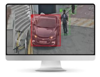
Using deep learning analysis technology, all-weather unexpected situations on the road (accidents, shoulder stops, etc.) are detected in real time, classified precisely, and provided to drivers and operators to prevent accidents in advance.
