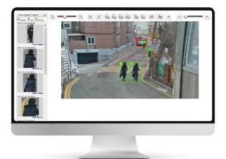
Object Detection technology allows operators to automatically identify and track target objects by using modeling technology that creates a fixed background in the scene, allowing the detection and monitoring of moving objects across the top.
