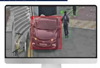
Using deep learning analysis technology, all-weather unexpected situations on the road (accidents, shoulder stops, etc.) are detected in real time, classified precisely, and provided to drivers and operators to prevent accidents in advance.
