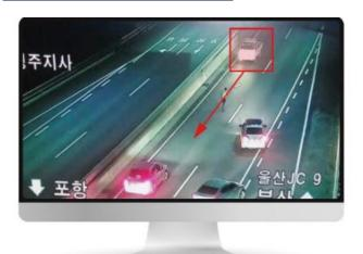
Reverse driving vehicle prevention system. Reverse driving vehicle prevention on one-way roads.
