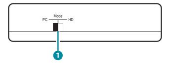
1 PC/HD switch: Press this button to switch input source between composite or S-Video. The Led will illuminate in yellow when switch to composite input and red when switch to S-Video input.
