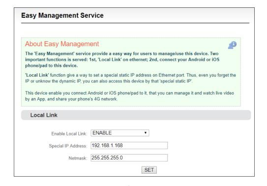
Localized connection" is to bind the encoder to a separate IP address, this IP address does not affect the use of other network cards, in special cases, it can play a role to manage encoder, this address can be manually changed, and the default address is 192.168.1.168.
