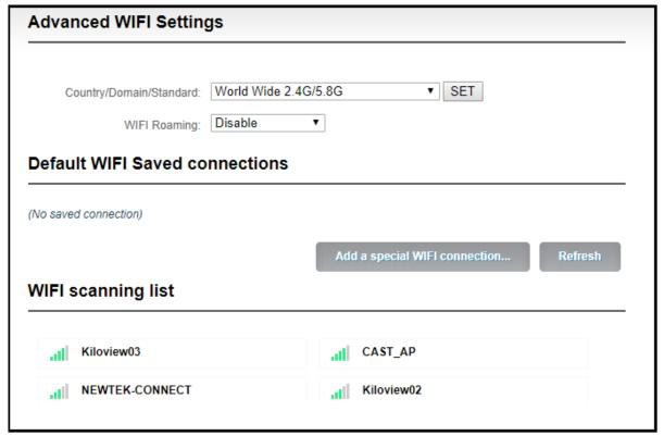
Note: In order to reduce the wireless network interference and obtain a good video playback experience, it is recommended to place the WIFI router and encoder in the visible range and connect the encoder to the 5.0GHz of the WIFI, and set the router to a relatively clean channel. In order to make sure the fluidity of the video while streaming with WIFI, the coding rate can be appropriately reduced as necessary.
