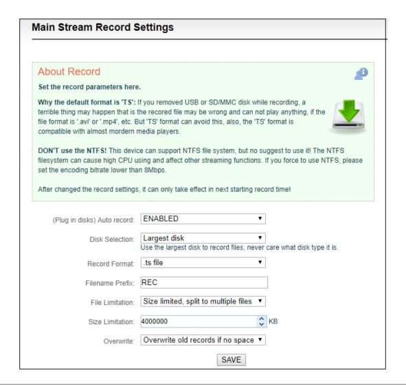
Note: A real challenge for recording by removable disks: If you remove the storage disk while recording, the recorded file may be wrong and can not be played if the file format is '.avi' or '.mp4', etc. But 'TS' format can avoid this, also, the 'TS' format is compatible with almost all the main media players.
