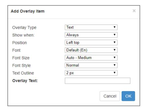
For every overlay, you can set the terms of overlay, position, font and font size, Image or text content and so on. After adding that, it will be shown as follows:
