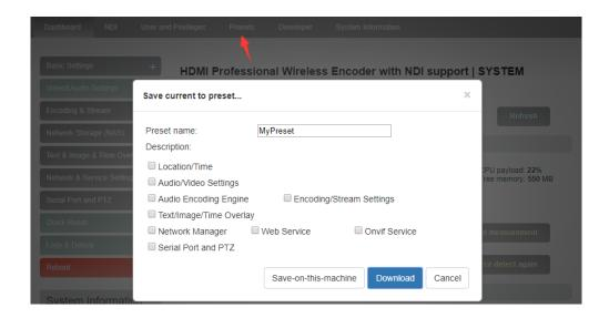
When there are other devices on site or the parameters of your device are restored to the factory, you want to use the parameters previously set. You can upload the saved configuration file in "manage or load preset configuration", restart the device after loading, and the parameter configuration will take effect.
