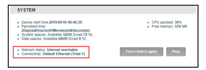
Note: Please confirm whether USB 4G card enables dial-up connection function, SIM card is workable, otherwise the network maybe unavailable. Users can insert a USB 4G card into a computer to test whether it can provide Ethernet access function.
