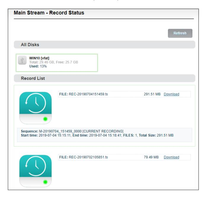
When it is recording, users can stop the recording manually and it can be restarted again.
