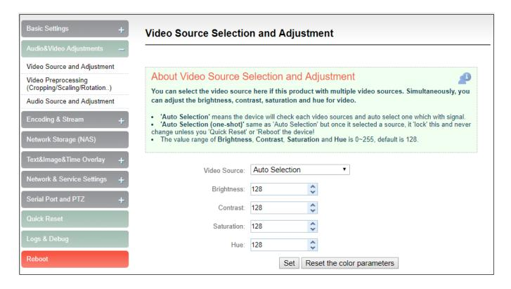
"Auto Selection" means the device will check each video source and automatically select the one which has signal.
