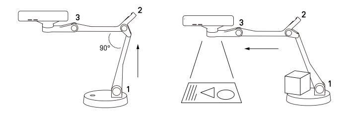
Uplift allows one-hand operation when its arm is partially folded. To remove your phone, please tilt it in one direction, until it is released from the magnetic holder.
